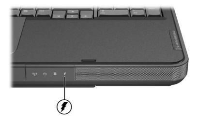
It is recommended that you leave the notebook connected to external power until the battery pack is fully charged and the battery light is turned off.
